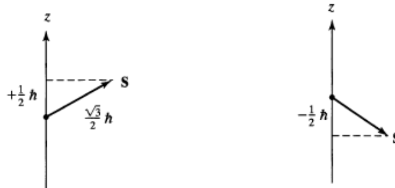
FIGURE 10.1 Possible orientations of the electron spin vector with respect to the z axis. In each case, \mathbf{S} lies on the surface of a cone whose axis is the z axis.
