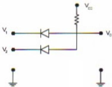
Diode based Logic
