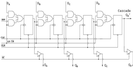
74LS395 parallel-in/ parallel-out shift register with tri-state output
