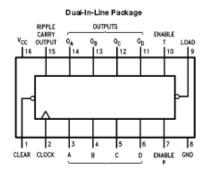
DM74LS193 Synchronous 4-Bit Binary Counter with Dual Clock
