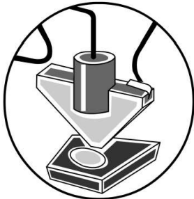
Schematic of the first transistor developed in Bell labs
