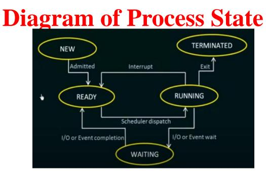
•In the next case that can occur is there can be a interrupt when the process was being executed.
