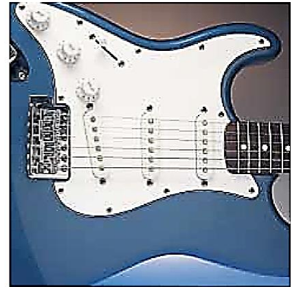
Fig. 4: (a) In an electric guitar, a vibrating string induces an e.m.f in a pickup coil. (b) The circles beneath the metallic strings of this electric guitar detect the notes being played and send this information through an amplifier and into speakers.
