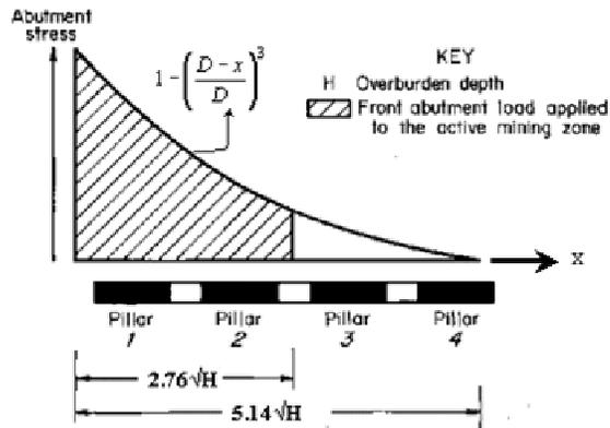
From experience and from numerical analysis it is found that the front abutment load reaches to zero at a distance given by the following equation  $D = 5.14\sqrt{H}$
