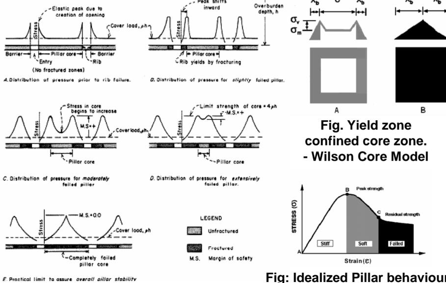
Fig. Yield zone confined core zone. - Wilson Core Model
