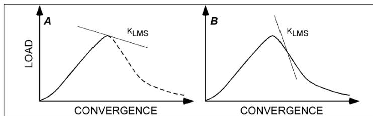
**Fig.—Unstable violent failure versus stable nonviolent failure. A, Unstable failure in a soft loading system. Loading machine stiffness is less than post-failure stiffness.**
