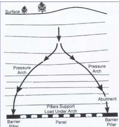
Fig. Yield Pillars – Pressure Arch Concept
