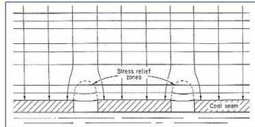
Fig. Pillar – Pressure Arch Concept
