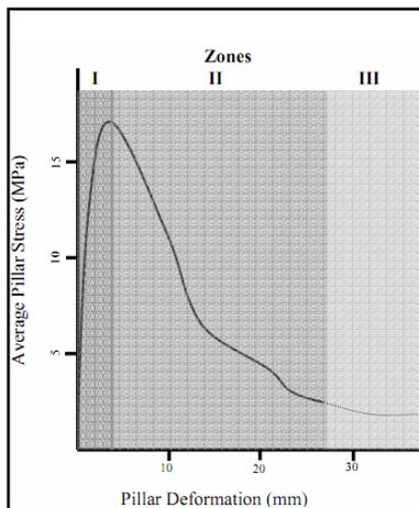
**Fig; Load Deformation Curve of a Coal pillar**
