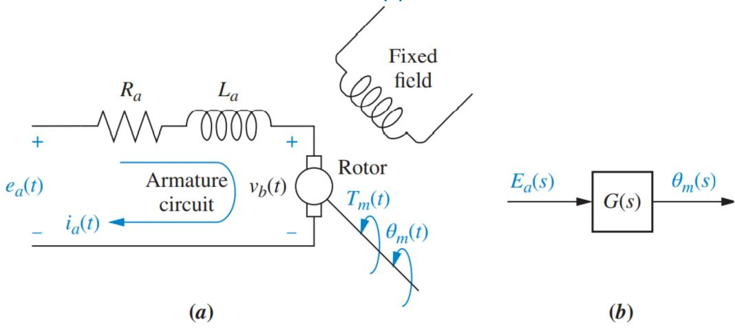
**2.35** DC motor: **a.** schematic; 12 **b.** block diagram
