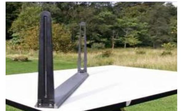
**Centering:** Centering is an essential step in plain table survey. The centering means to set the table vertically on the ground point.
