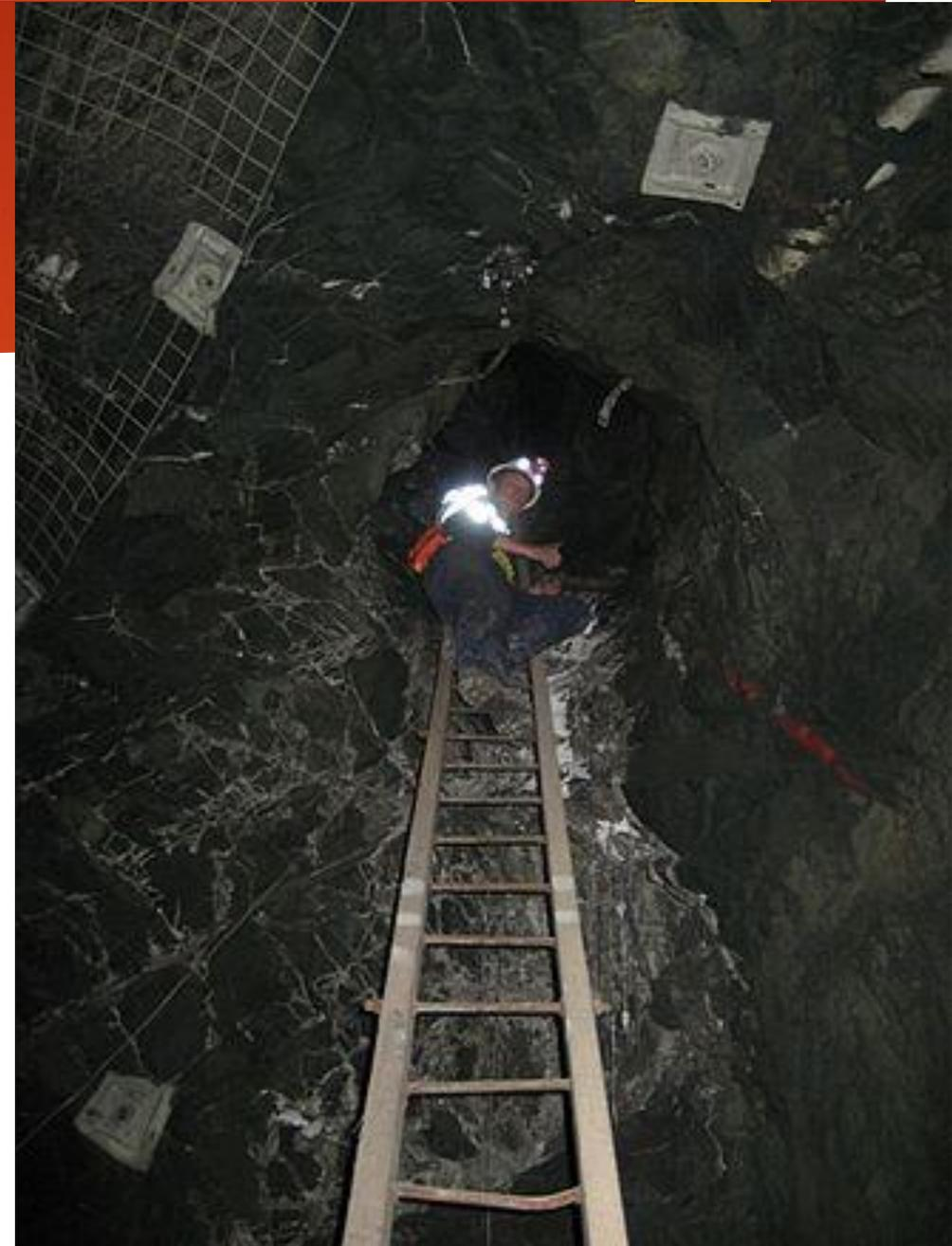
Raising is a difficult and dangerous, but necessary job. Raising methods vary from simple manual drill and blast to mechanical rock excavation with raise boring machines (RBMs)
