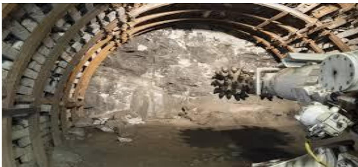
The primary opening into an underground mine to provide access for people, materials, and equipment and to enable the ore to be brought to surface can be a shaft sunk vertically or on an “incline”; a “decline,” which is a ramp driven into the earth usually in a spiral fashion; or an “**adit**,” which is a main horizon/main access opening.
