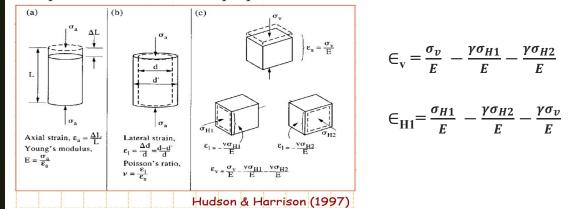
To provide an initial estimate of the horizontal stress, two assumptions are made-
