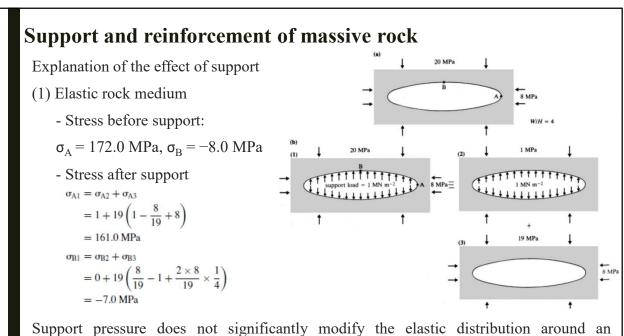
Support pressure does not significantly modify the elastic distribution around ar underground opening
