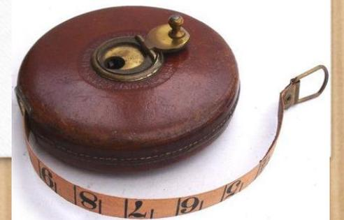
**Metallic Tape:** It is a linen tape with brass or copper wires woven into it longitudinally to reduce stretching. As it is varnished, the wires are not visible. These are available in 20-30 m length. As it is reinforced with wires, all the defects of linen tapes are overcome.
