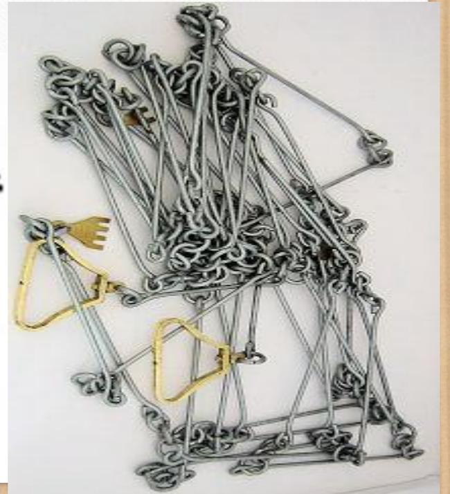
**Metric Chains:** Metric chains are generally available in lengths of 5, 10, 20 and 30 metres. To enable the reading of fractions of a chain without much difficulty, tallies are fixed at every metre length for chains of 5 m and 10 m lengths and at every five-metre length for chains of 20 m and 30 m lengths.
