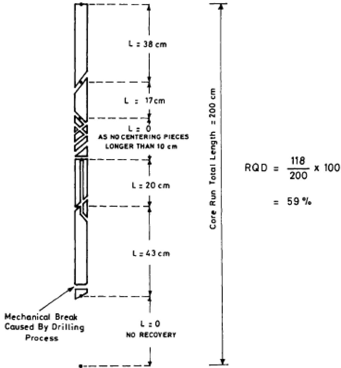
Figure 4.1: Procedure for measurement and calculation of rock quality designation RQD (Deere, 1989)
