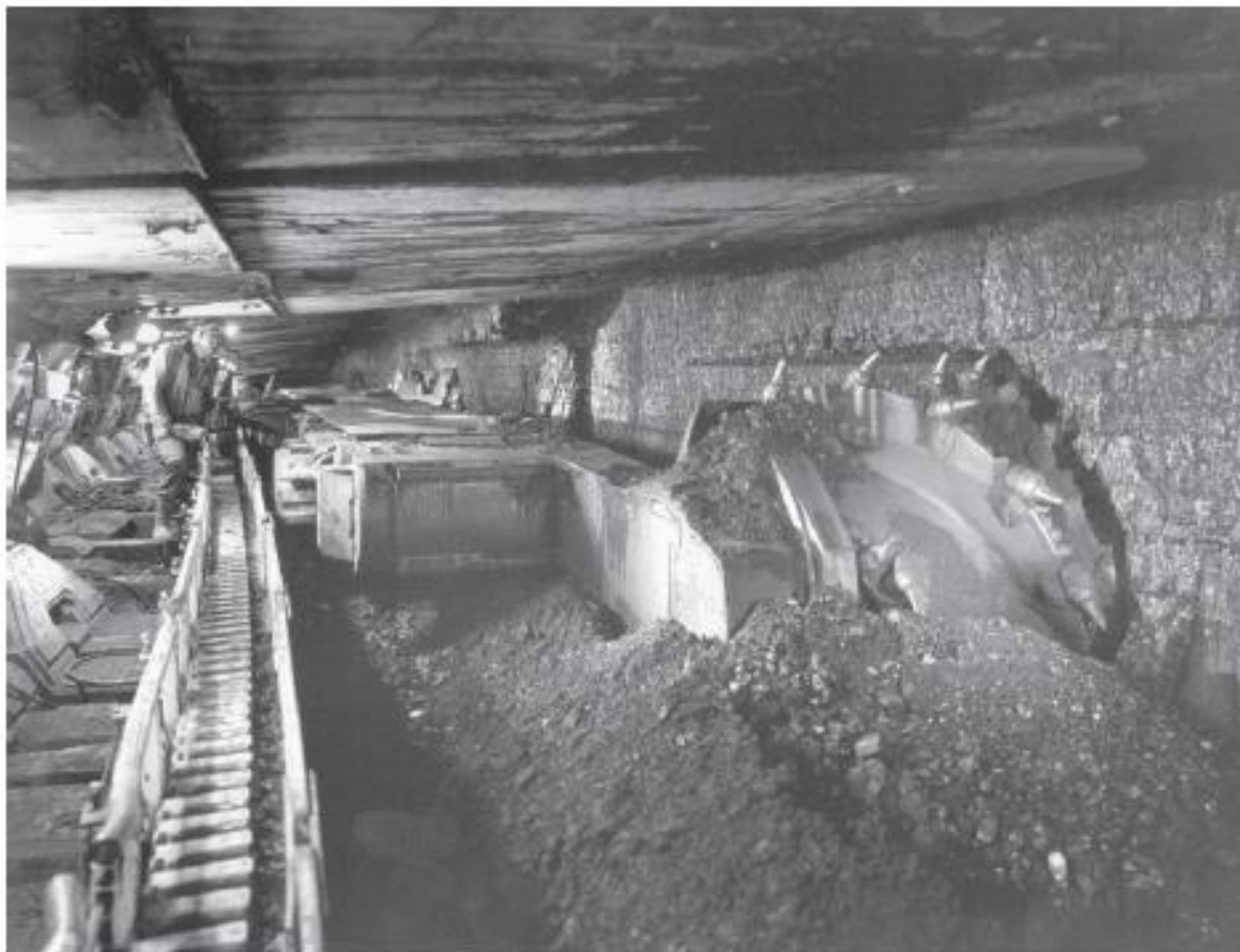
FIGURE 3-7 Photograph of longwall coal mining. SOURCE: CONSOL, Inc. (now CONSOL Energy, Inc.)
