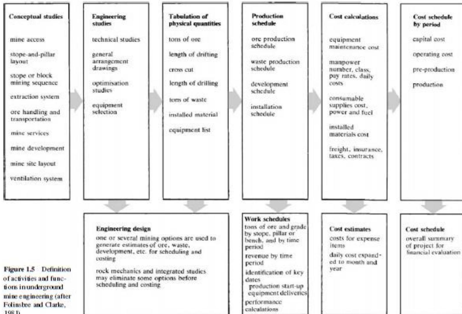
**Figure 1.5** Definition of activities and functions in underground mine engineering (after Folinsbee and Clarke, 1981).
