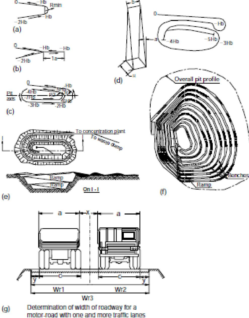
Figure 17.6 (a) to (e): Haul road's and ramp designs for surface mines. Ramp designs: Spiral, Shunt-back and, Combination. (g): Determination of haul-road width;  $a = T_w =$  truck width; Also  $a = c$ ;  $c$  is out-to-out tyre width of truck.
