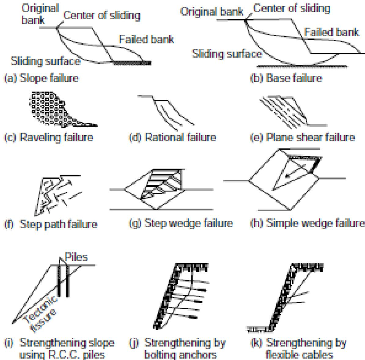
Figure 17.4 Open pits' common failure patterns (a to h), and common slope strengthening techniques (i to k).
