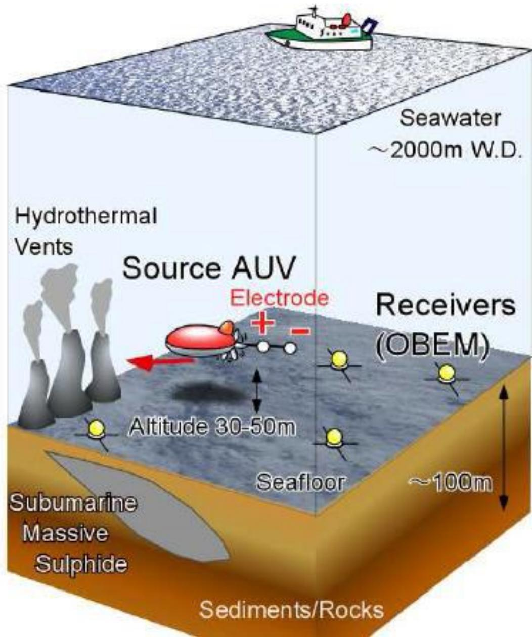
In a similar way to CSEM surveying, the MT technique is sensitive to resistive bodies in the subsurface. Marine MT surveys map subsurface resistivity variations by measuring naturally occurring electric and magnetic fields on the seabed.
